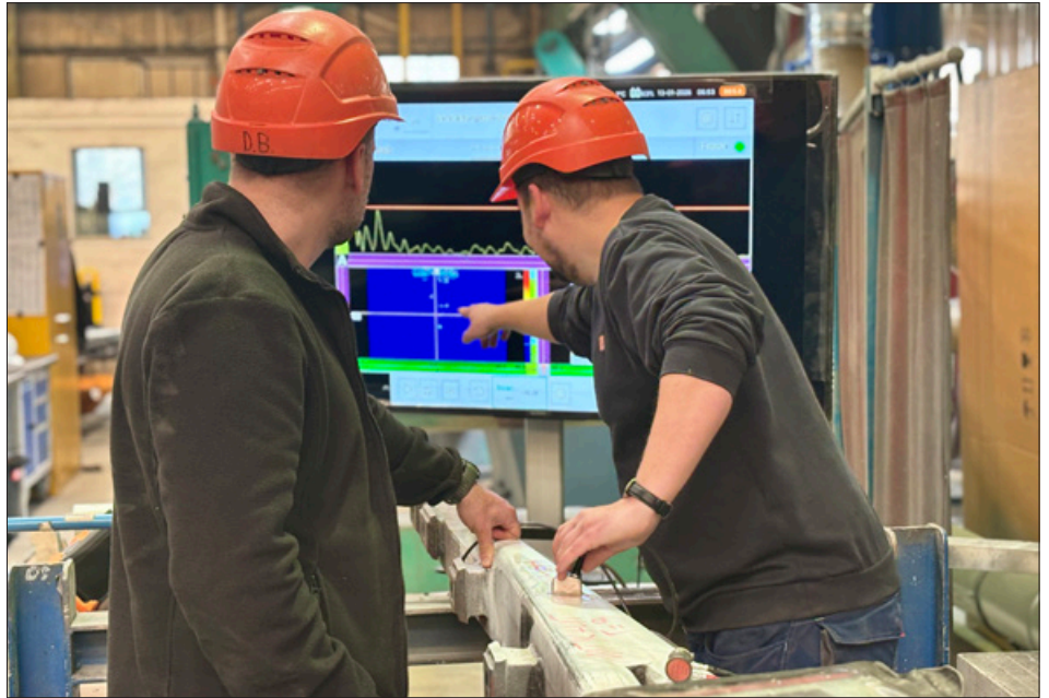
A modern test station, equipped with a TFM testing instrument and a probe from KARL DEUTSCH, built to the customer's specifications
