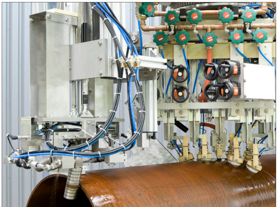
Example system: ECHOGRAPH SNUS for ultrasonic testing of the weld, the pipe end and the heat-affected zone
