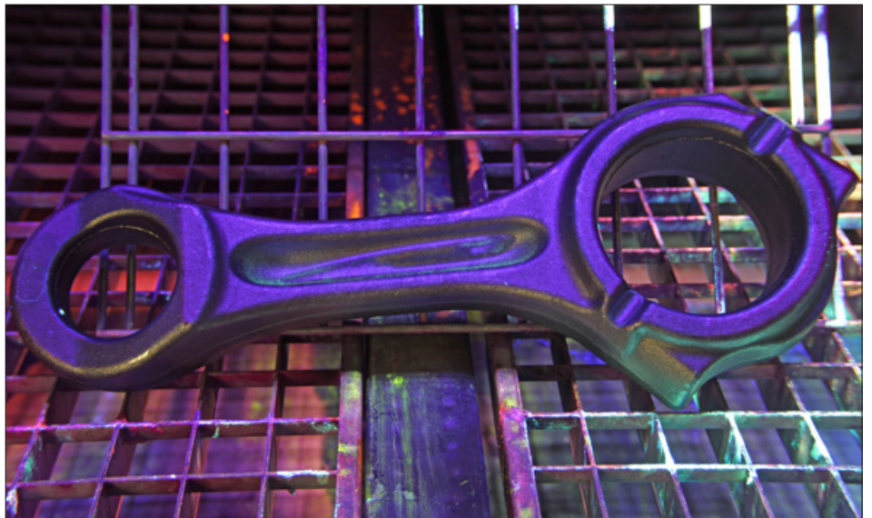
Connecting rod cleaned with KD-CHECK PREW-AS
