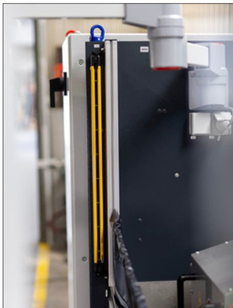
Light barrier with three functions: Cycle start, prevention of pinching hazards and counting of test parts
