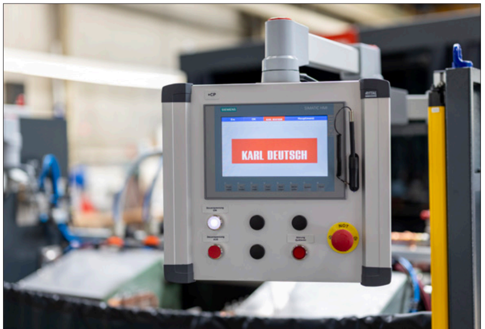
Convenient: During setup, the control panel can be swivelled directly next to the test area without triggering the light barrier
