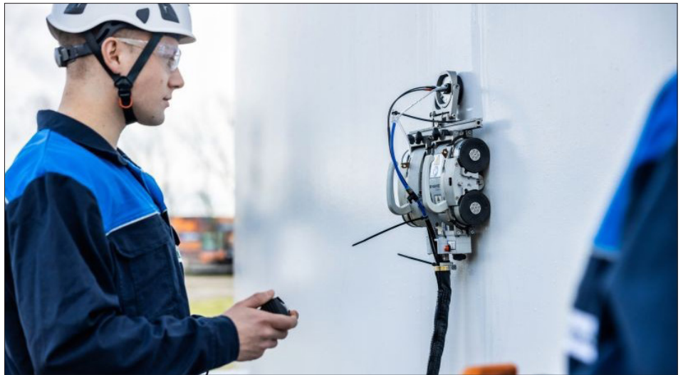
Efficient testing on the tank wall: NAVIC 2 with GEKKO in PAUT mode (130 mm/s)
