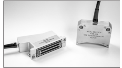
Examples of phased array probes for bar testing, manufactured with up to 128 elements in various radii of curvature and test frequencies
