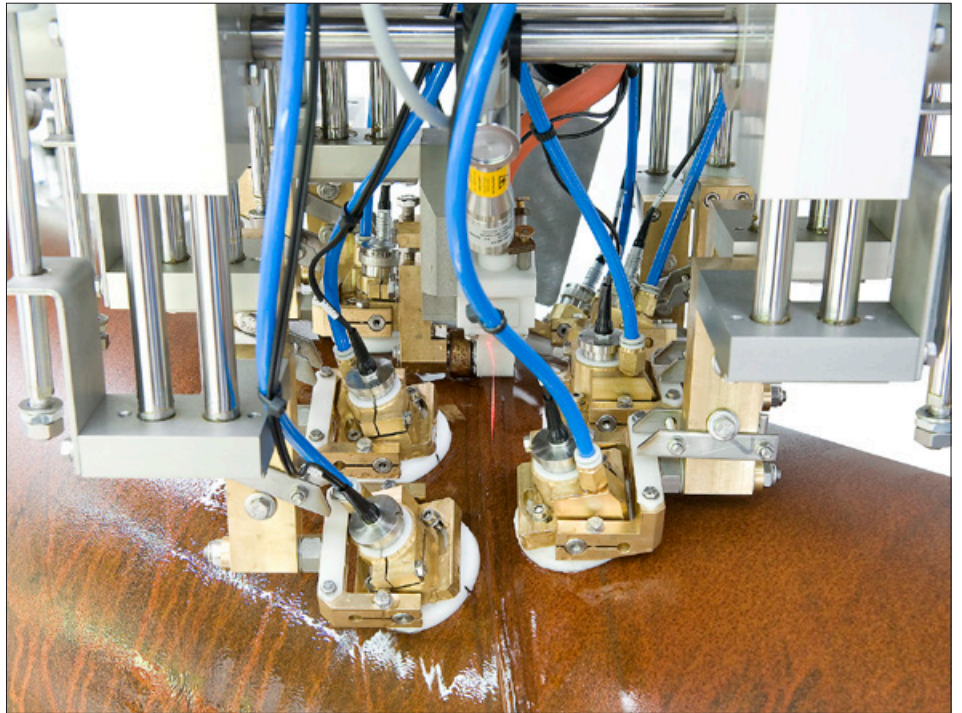
Example of the ECHOGRAPH SNUS probe holders with automatic seam tracking
