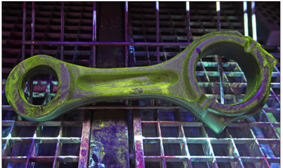
Uncleaned connecting rod with magnetic powder residue
