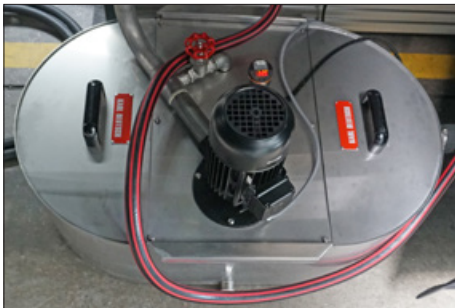
Container for testing medium with sensor for monitoring of the test medium temperature
