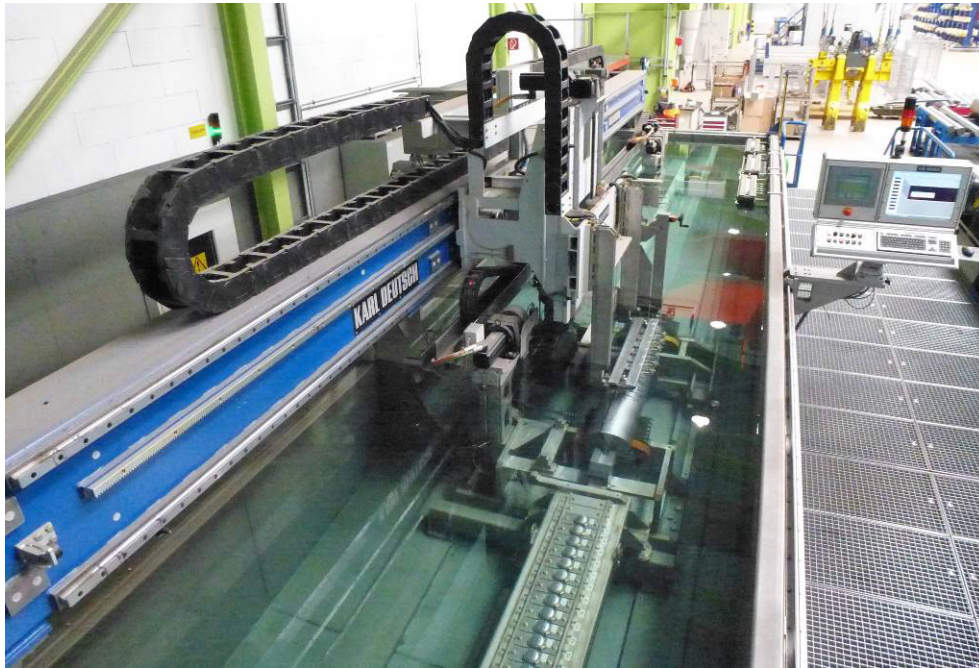
Figure 1. Total view of immersion tank testing system for aerospace bars at the VDM Metals GmbH workshop in the town of Unna, Germany.
