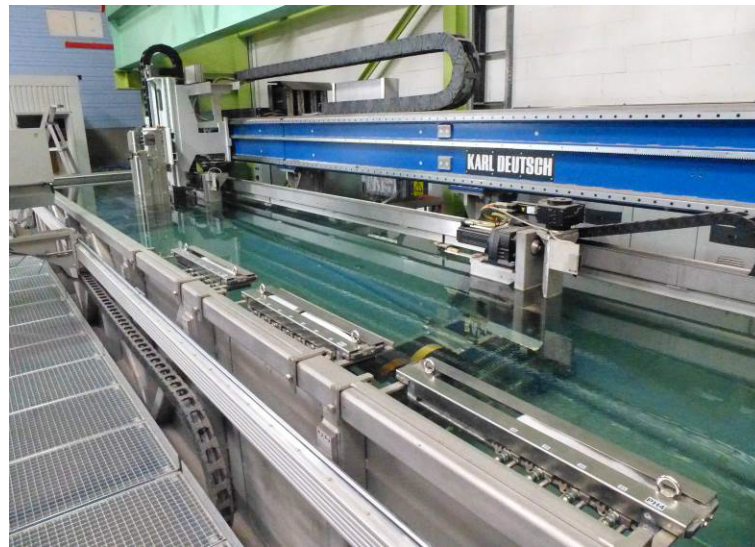
Figure 5. The testing system was equipped with four probe holders, which can be changed by quick-release fixtures. Three probe holders which are currently not in use can be seen in the foreground of the photograph.
