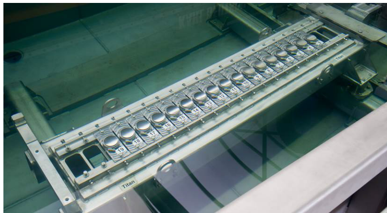
Figure 7. A test block fixture at the base position of the tank is used for periodic check of the test sensitivity in intervals of two hours.
