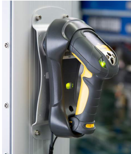
Figure 13. Barcode-scanner for error-free bar tracking during the production and testing process.
