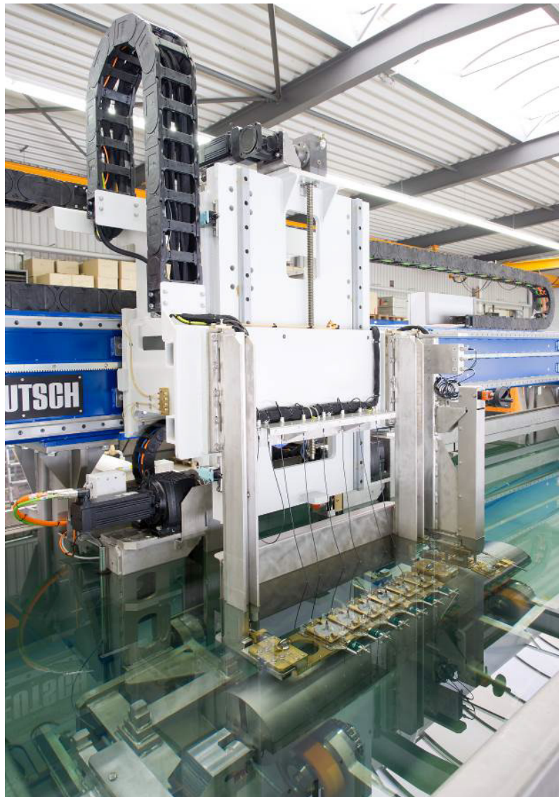
Figure 2. Probe holders above a calibration bar with a length of 1.5 m. In case of short bars, only two out of three roller stations are used. The rubber-coated rollers avoid damaging of the bar surfaces.
