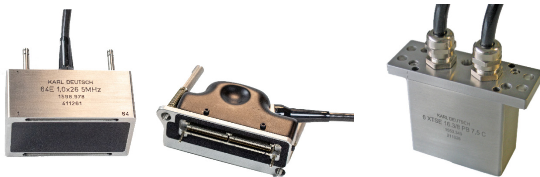
Fig. 3. Probes used in the system. Left: Phased array probe, right: Multi-transducer TR probe.
