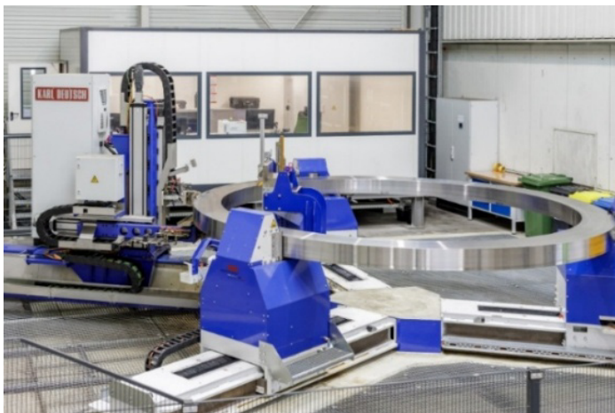
Fig. 2. The testing system contains three roller blocks (A) and the carriage with the mounted probes (B)
