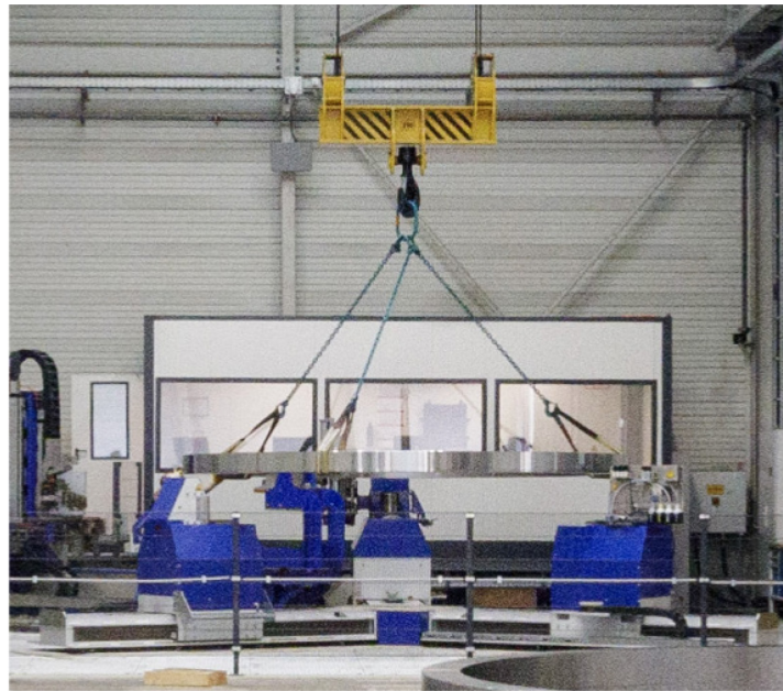
Fig. 1. Loading of the rings into the testing system
