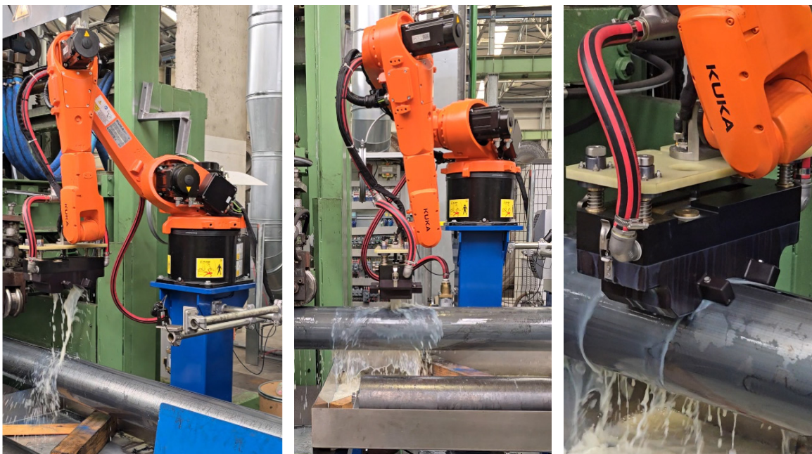
Fig. 6. Water gap coupling of PAUT probe
