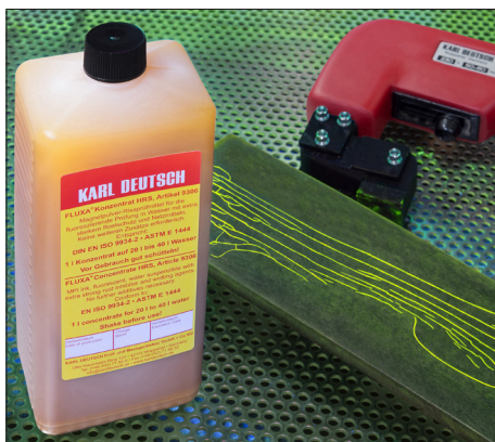
FLUXA: Agents for magnetic particle testing
