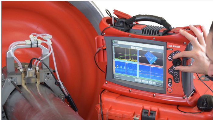
WS3: Semi-automatic inspection of wheelsets. First, the axle is tested, then the wheel flange with a second phased array probe holder.
