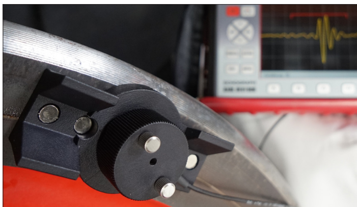
WS-RS: The residual stress is determined with an ultrasonic flaw detector with extremely precise time-of-flight measurements and a custom probe.
