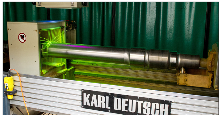
DEUTROFLUX UWS: Cabin ceiling enables crane loading from top.
