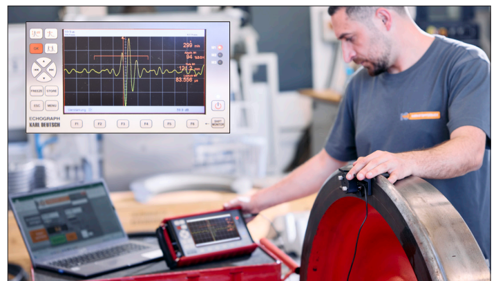
WS-RS: The residual stress is determined with an ultrasonic flaw detector with extremely precise time-of-flight measurements and a custom probe.
