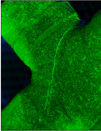
Crack indication with fluorescent magnetic powder
