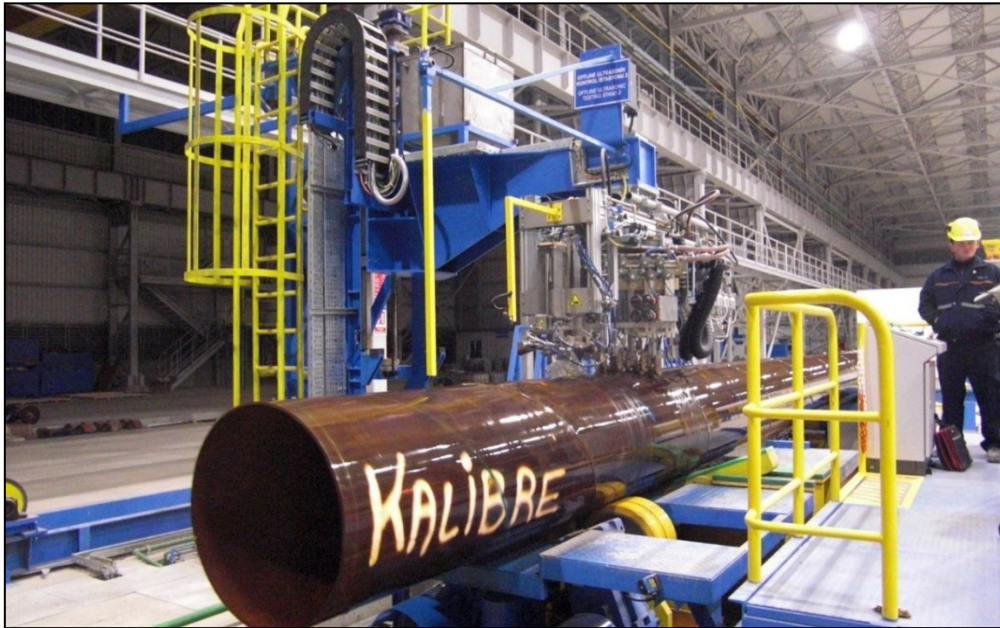
Fig 14. HSAW-pipe weld testing using horizontal boom and pipe carriage.
