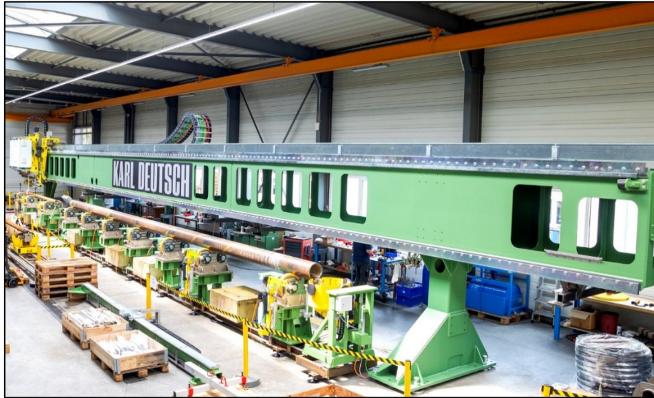
Fig 4. Testing bridge for pipe inspection before shipment. The pipe to be tested is positioned on a set of double rollers. The yellow testing carriage is linearly moved along the rotating pipe.
