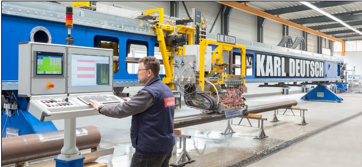
Fig 12. Testing bridge for offline ERW-pipe weld testing (before shipment). The yellow test carriage is travelling along the pipe at a high speed. A calibration station is on the left.
