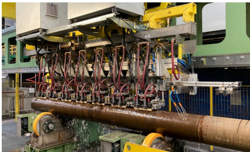
Fig 5. Inspection of black pipes with seven probe holders. The diameter range was 60 – 270 mm, the wall thickness was up to 50 mm and oblique defects up to 75° were detected.
