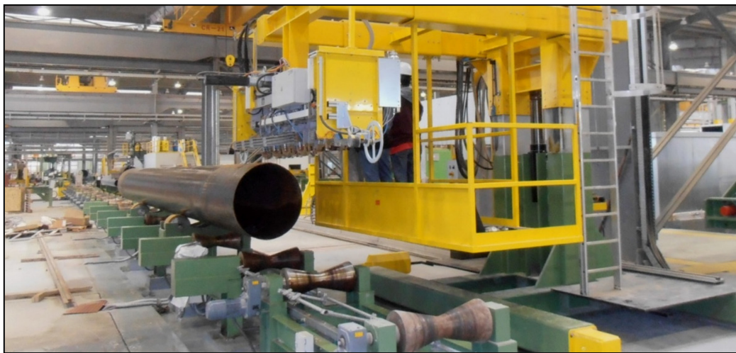
Fig 16. LSAW-pipe weld testing with horizontal boom and pipe carriage
