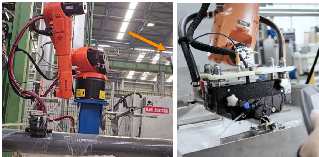
Fig 11. Online ERW-pipe weld test using a robot (left), dynamic sensitivity check on calibration tube (right).
